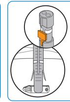
2) Press the plunger down until the plunger's white line meets the top of the orange stopper. You will see the needles partially exit M-Close without entering the tissue
